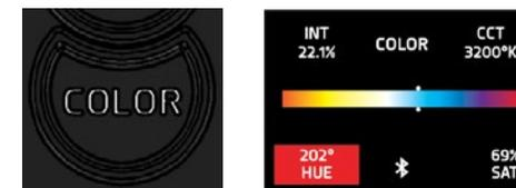
Color selection mode. This mode is an HSI (Hue, Saturation, Intensity) with the ability to select the white base between 1700°K and 10000°K.
