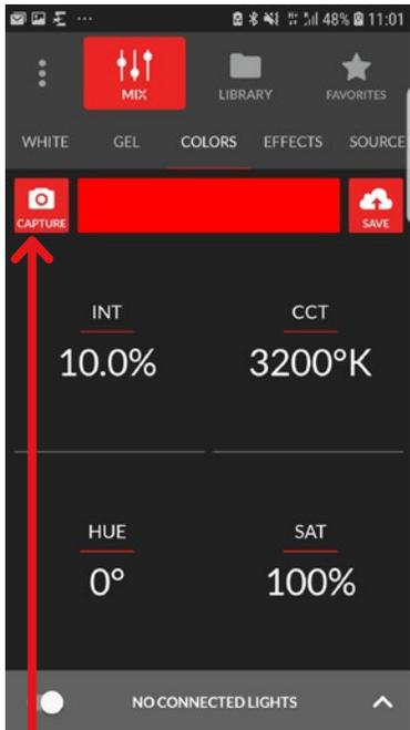
In the color mode, touch the camera to access the CAPTURE function.
