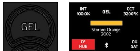
Gel selection mode where you can select any of the gels available in the MIX (standard and saved). Saturation and hue are available on a limited range.
