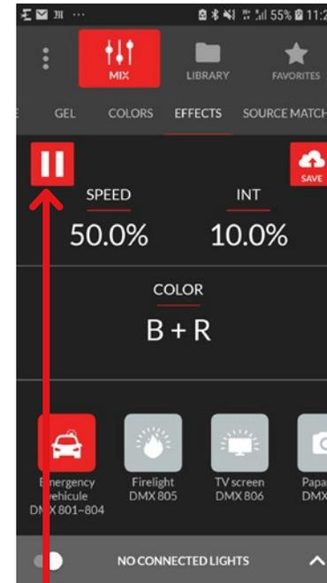
Effect Mode: press the PLAY button, select the effect, change speed, intensity and the color of the LEDs.
